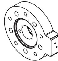
MOUNTING INTERFACE FOR DIRECTIONAL CONTROL VALVE\* TO: ISO 4401 SIZE 03/ANSI B93.7M SIZE D03
